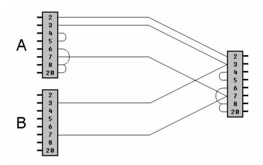
All ends are terminated with 25-pin male RS-232 connectors. Jumpers are required on two of the three connectors as shown.
